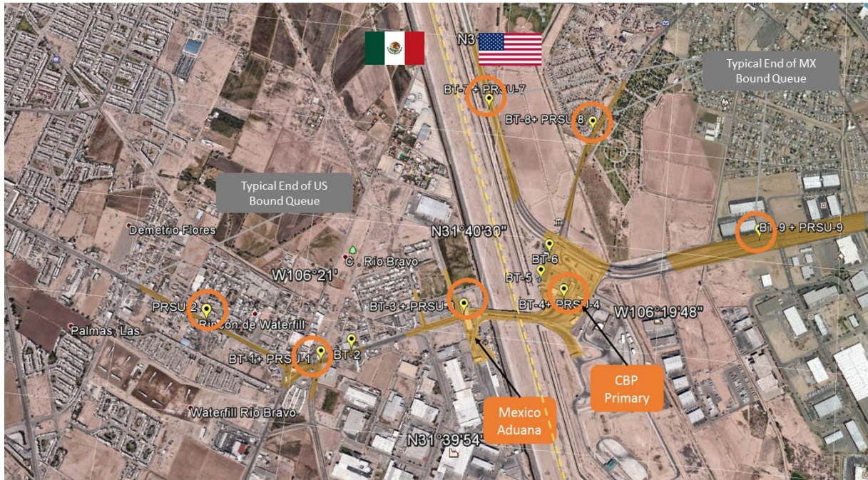
Figure D-10. Aerial Image of Ysleta-Zaragoza POE Showing Existing Locations of Bluetooth Sensors and Potential Locations of DSRC Sensors.
