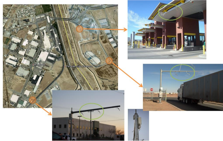
Figure 5. RFID Technology–Based System to Estimate Wait Times of COVs at Ysleta-Zaragoza POE (Source: Texas A&M Transportation Institute [TTI]).
