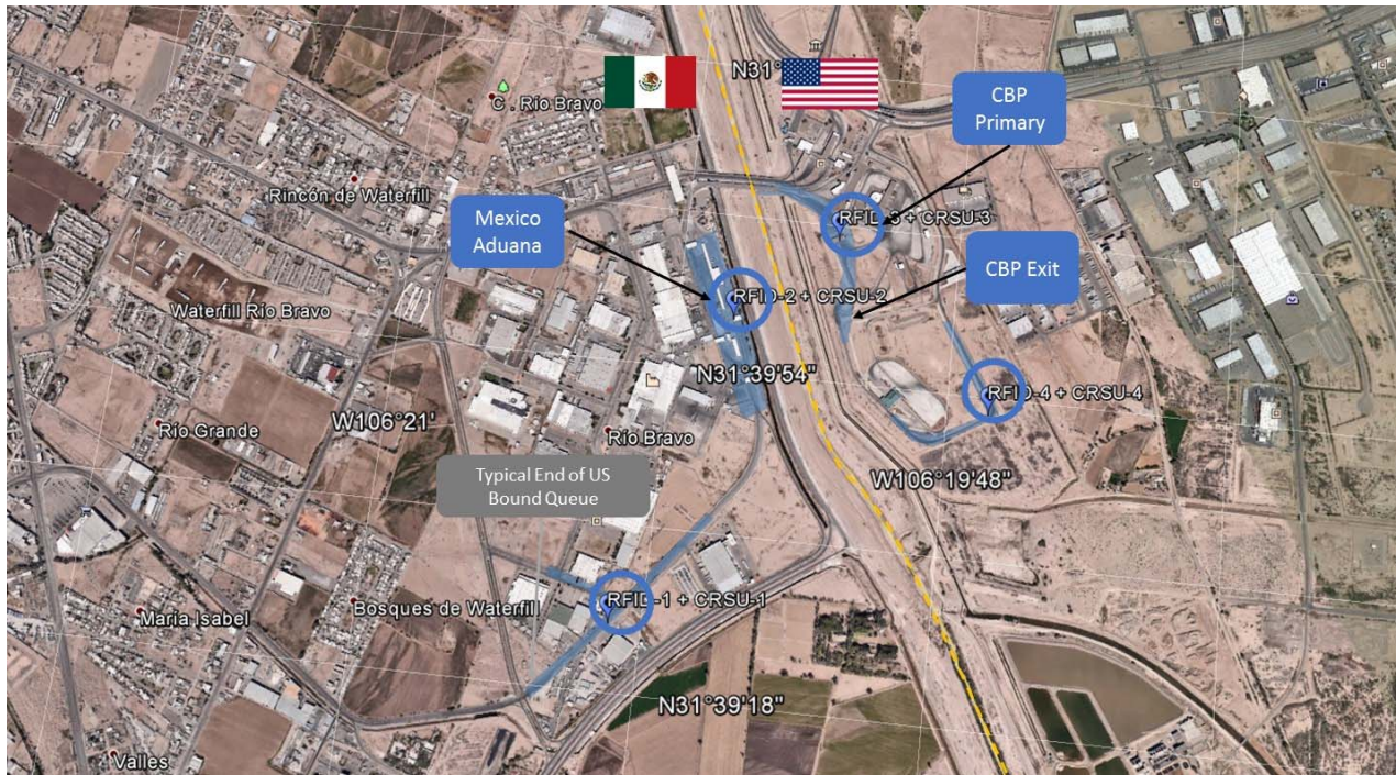
Figure D-11. Aerial Image of Ysleta-Zaragoza POE Showing Existing Locations of RFID Sensors and Potential Locations of DSRC Sensors.
