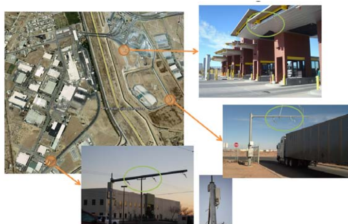
Figure D-2. RFID Technology–Based System to Estimate Wait Times of COVs at Ysleta-Zaragoza Port of Entry (Source: Texas A&M Transportation Institute [TTI]).
