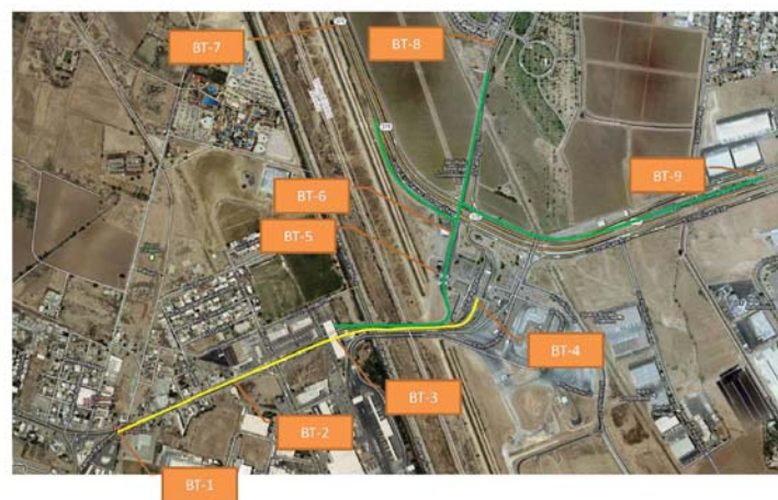
Figure D-3. Bluetooth Technology–Based System to Estimate Wait Times of POVs at Ysleta-Zaragoza Port of Entry (Source: TTI).
